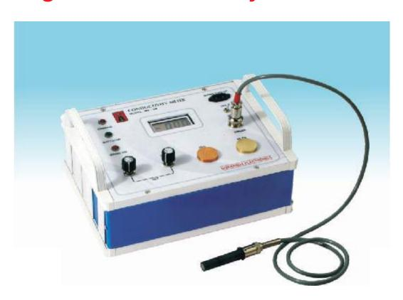
Portable Conductivity Meter has been developed to facilitate easy determination of conductivity of non-ferrous metals based on eddy current principle. Instrument uses a probe which when placed on the surface of metal indicates conductivity on a linear scale panel meter.
