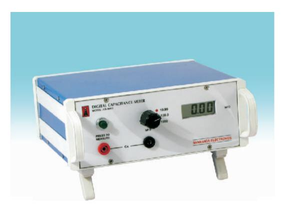
Digital Capacitance Meter LS 16 AD is specially designed for accurate measurement of Capacitance. It is portable and easy to carry. Test frequency used is 120 Hz, which allows error free measurement. 3½ digit LCD DPM displays the Capacitance value. Test leads can be plugged into Cx sockets. Suitable range can be selected through selector switch. Reading will be displayed on DPM after pressing push button provided on front panel.
