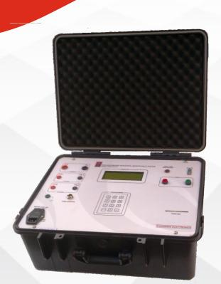
TRANSFORMER WINDING RESISTANCE METER
