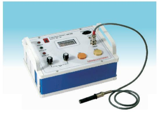
Portable Conductivity Meter has been developed to facilitate easy determination of conductivity of non-ferrous metals based on eddy current principle. Instrument uses a probe which when placed on the surface of metal indicates conductivity on a linear scale panel meter.
